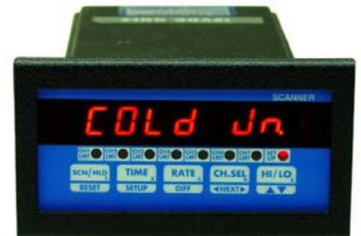
**NOTE 1:** The unit must be powered up for at least ten minutes before adjustments are made to cold junction reading.
