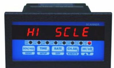
digit. Pushing ^v key and keeping it pushed, will increment the digit. Releasing ^v key and then pushing it again will decrement the value (^v key works as a toggle -- alternating between increment and decrement). To change the next digit first push the <NEXT> key. This will advance the flashing to the following digit. Use ^v key to change the value. After the desired High Scale setting is displayed, push **SETUP** key to enter that setting and go to setup Low Scale.
