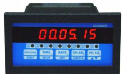
The elapsed time can also be momentarily displayed while the unit is operating in any other display mode. This is done by pushing the **TIME** key once. The unit will first display the word 'ELPSd t' followed by the elapsed time. This will stay in the display window for a brief period and then the unit will revert to the normal display mode.
