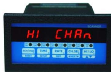
To display high and low channel from any other display mode simply push the **HI/LO** key. Pushing this key once will first display **'HI CHAN'** and then the channel number and the process value will be displayed in the format **'C2 1234'**. The second push on the **HI/LO** key will first show **'LO CHAN'** in the display window, and then the channel with the lowest process value will be displayed.
