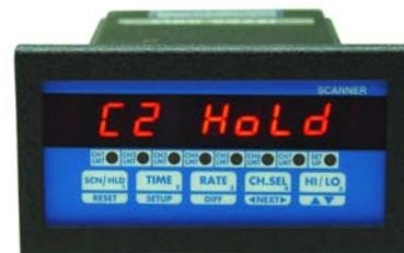
To select another channel for display during hold mode, push the **CH. SEL** key. Each push will increment the channel number. The display will first show the channel number (e.g. **'CHANNEL 2'** for channel # 2) followed by the process variable in the form **'0.123 PSI'**. When channel selection is initiated using the **CH. SEL** key, the unit starts with channel #1 and steps thru to channel #7 with each push of the key.
