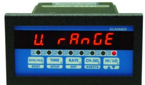
may be setup. The display will briefly show 'U rAnGE' (for "Voltage Range") followed by the current setting. Use ^v key (ref. Setup For High Scale) to set the desired VOLTAGE value. Once the desired value is displayed, push SETUP key to enter that value and go to the next step.
