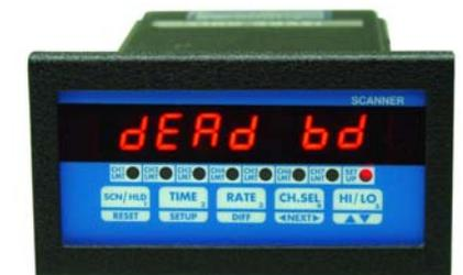
The display will first show 'dEAd bd' after which present DEADBAND value will be displayed. Use ^v key (ref. Setup For High Scale) to set the desired DEADBAND value. Once the desired DEADBAND value is displayed, push SETUP key to enter that value and go on to setup Relay as Normally Open/Closed.
