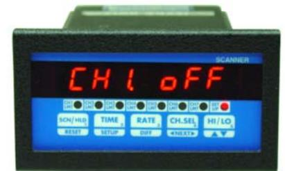
Use ^v key to display the desired ON/OFF setting, and then push SETUP key to enter that setting and go on to setup Decimal Point Position.
