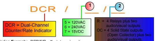
**Ordering Example:** DCR/5/R -- Dual channel monitor with Pulse inputs, 120vac Power and relay output option.
